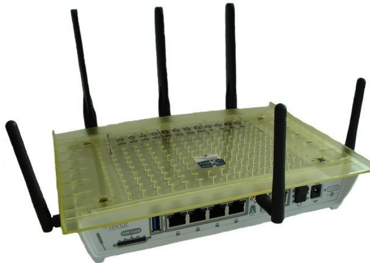
Figure 6: Perspective view of Teldat-K router (with WLAN and WWAN antennas)
