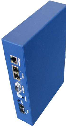
When Rail mounting is a requirement the FlexDSL Orion 2 Repeater with DIN Rail case is the right choice, extending single pair SHDSL (TC-PAM16/32) up to 5.7Mbps. it offers Ethernet add/drop functionality (10/100BT, Bridge) and comes in a blue (RAL 5003) powder coated metal housing with white labeling.
