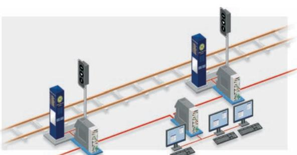
LineRunner SCADA NG transmits different application data simultaneously over a transmission route. Video and control data can be transmitted via RS-232 and Ethernet at the same time.
