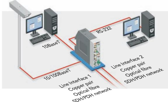
Three user interfaces are available for each LineRunner SCADA NG. A serial interface for low bandwidths and two Ethernet interfaces for large volumes of data. In each LineRunner SCADA NG with exchangeable line interfaces you can implement the change from one transmission medium to another.
