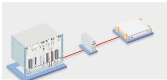
LineRunner SHDSL DTM is the compact new network termination for leased lines with the Multi-Service Access Multiplexer UMUX. A maximum of 128 leased lines can be multiplexed on one STM-4 interface. Combine UMUX and LineRunner SHDSL DTM for highly flexible SHDSL transmission networks for a variety of applications. For further information on the UMUX family please refer to the UMUX product information.
