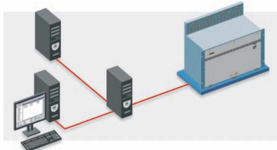
LineRunner ASMOS Pro is designed to manage even large networks. ASMOS server and the data base can be distributed on two PCs. Up to 10 ASMOS clients can access the modules at the same time. All accesses are managed using Microsoft® COM/DCOM. An extensive system of access rights protects your application against unauthorised access.
