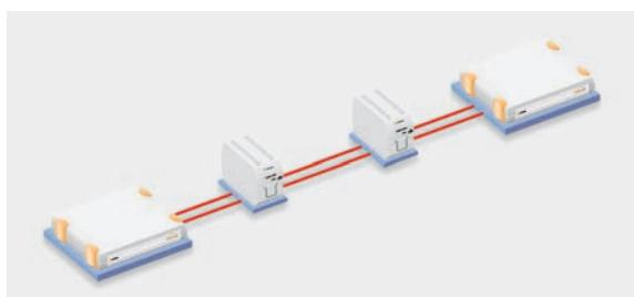
A maximum of 2 regenerators (with complete management capability and remote supply) can be integrated in the transmission routes. The outdoor housing is prepared for installation of LineRunner transmission technology even in the toughest of environmental conditions.
