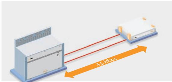
LineRunner SHDSL LCM/DTM provides you with a bandwidth of max. 4.6 Mbps via the optional Ethernet application interface.
