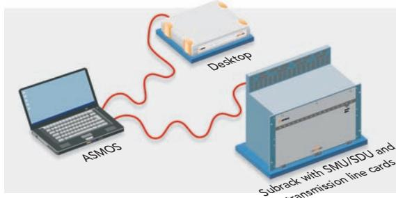
Configure modules on site locally with LineRunner ASMOS CT. Installed on a laptop you can access modules via the Ethernet RS-232 interface. Even local access to subracks via an SMU/SDU is possible.
